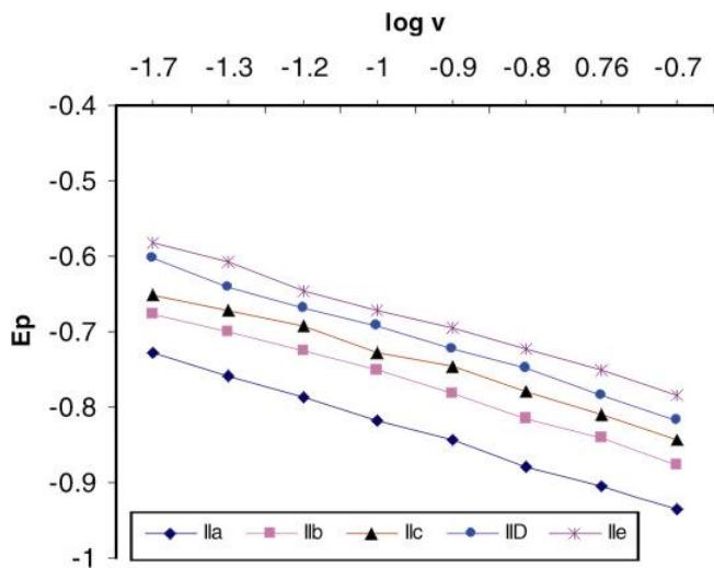
**Figure 3.** Plot of peak potential vs log of scan rate for Schiff bases (IIa–e) at concentration 0.1 m mol.
