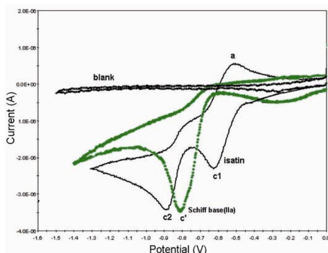
**Figure 1.** Comparative CVs of isatin and Schiff base (IIa) in DMF with aqueous 0.1 M LiCl as supporting electrolyte at HMDE at scan rate  $100 \text{ mV s}^{-1}$ , concentration 0.2 mmol.
