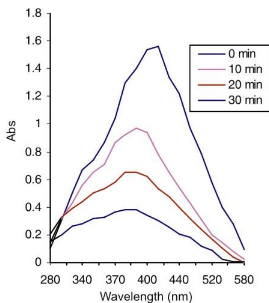
**Figure 4.** UV-Vis absorption spectra of compound IIa at different time intervals during constant potential electrolysis.
